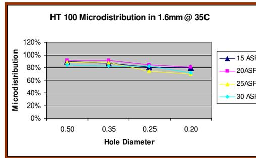
**Figure 11 – Microdistribution for 1.6mm Thick Panel Plated 35°C**
