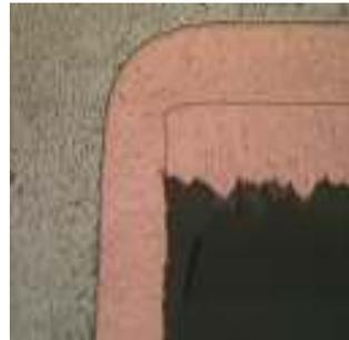
**Figure 12 – HT Process, Plating at 35°C, 2.0 ASD; Cross Section of 0.5 mm through hole after 6x Solder Shock**
