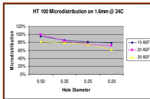
**Figure 10 – Microdistribution for 1.6mm Thick Panel Plated 24°C**
