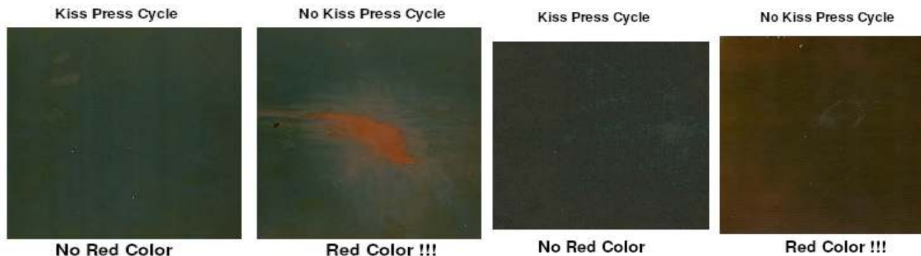
Fig 9 - One Drop of water added before lamination Fig 10 - 72 hours at 280C and 95% relative humidity
