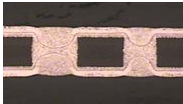
Figure 19. Two-step bridge & fill of TH's
