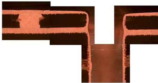
Figure 16. PCB via fill and TH plating
